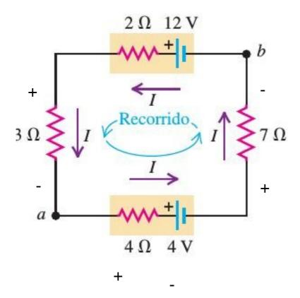
$$12v - I2\Omega - I3\Omega - I4\Omega - 4v - I7\Omega = 0$$
